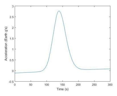
Figure 12. Acceleration profile of the probe during entry.
