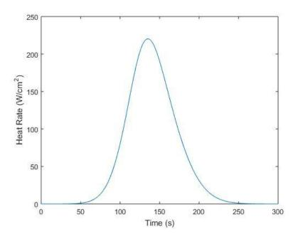
Figure 11. Stagnation point convective heating profile of the probe during entry.
