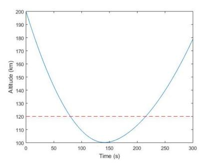
Figure 10. Altitude profile of the probe during entry.
