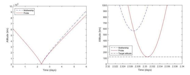
Figure 8. Mothership and probe altitude profile of the Venus flyby encounter.
