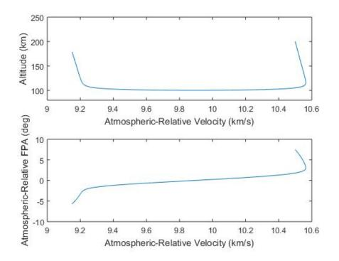
Figure 9. Altitude (top) and flight path angle (bottom) as a function of velocity.
