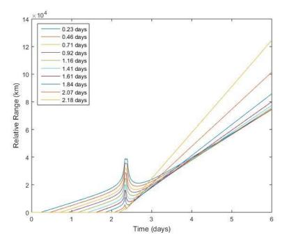
Figure 3. Time history of relative range between the probe and mothership during Venus flyby encounter for different separation times.
