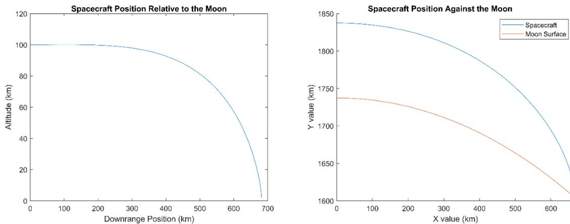
Figure 13. (a) Left: Spacecraft position in a 2-D sense as witnessed from the surface of the Moon. The downrange position is given in respect to a starting position of the Moon’s north pole. (b) Right: Spacecraft position given in the x-y coordinate system described earlier
