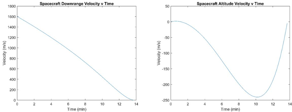
Figure 12. (a) Left: Spacecraft velocity as seen along the surface of the Moon, not in the x and y coordinate system. (b) Right: Spacecraft velocity vertically from the surface of the Moon throughout the length of the descent
