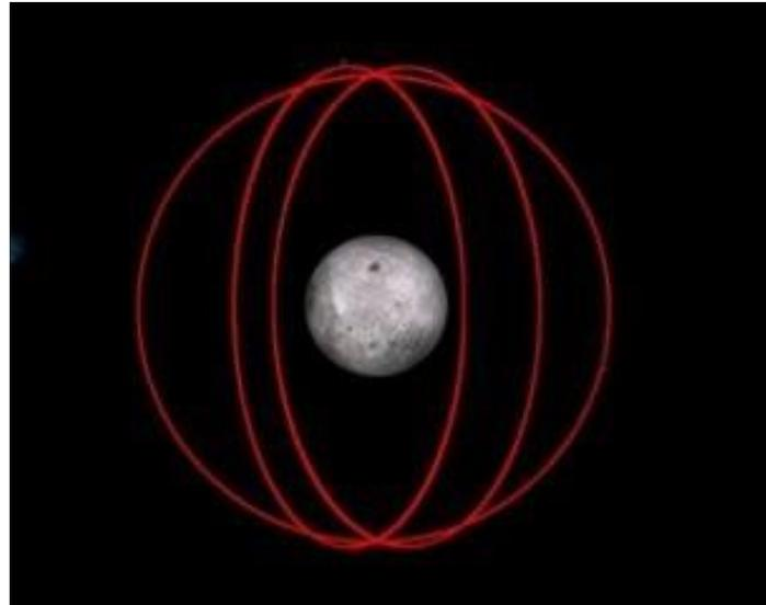
Figure 5. Proposed architecture for Lunar GNSS. Each of the planes will consist of 8 different satellites to obtain global coverage
