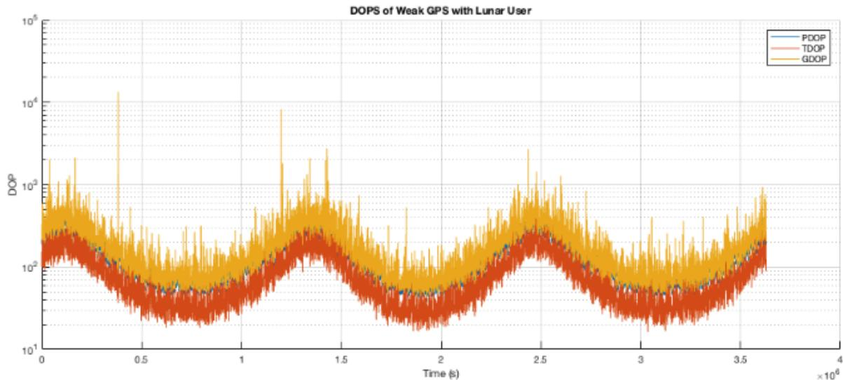
Figure 2. PDOP of Lunar Gateway in simulation for a duration of 50 days<sup>[4]</sup>
