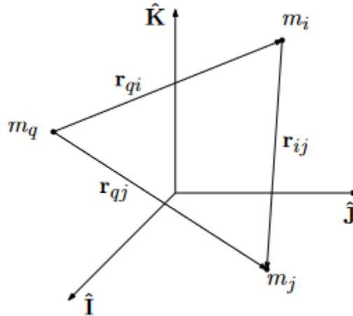
Figure 6. Definition of the geometry for the N-Body problem.<sup>[22]</sup>
