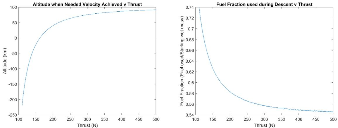
Figure 10. (a) Left: Final altitude of the spacecraft off the lunar surface when x and y velocities were under 5 m/s for various thruster forces (b) Right: Fuel fraction consumed in achieving the final position, compared to the starting mass of 100 kg. The fuel fraction was capped off at 0.74 to leave at least 0.26 for both the dry mass and controlled descent if needed.
