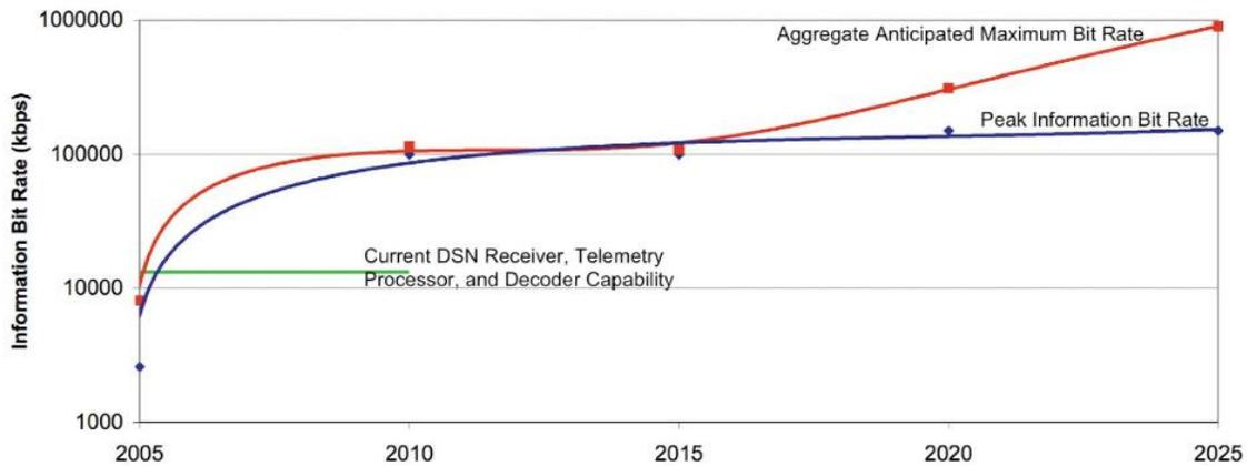
Figure 1. Projections of Needed Mission Downlink vs Current DSN Capabilities<sup>[1]</sup>
