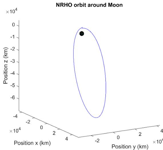
Figure 7. Simulated NRHO orbit from which the spacecraft could be deployed. The central body shown in the figure is the Moon
