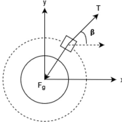
Figure 9. Diagram of the 2-body problem where the central body is the Moon, T resembles thrust, Beta is the thrust angle,  $F_g$  is the force of gravity, the dotted line resembles the spacecraft orbit, and the x-y axis belongs to the Moon centered, Moon-fixed reference frame.
