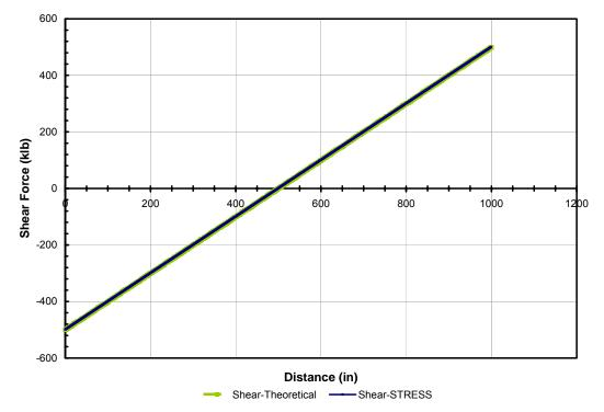
Figure 5. Shear Force Accuracy of Discretized vs. Theoretical Method for Uniformly Loaded Simple Support Beam
