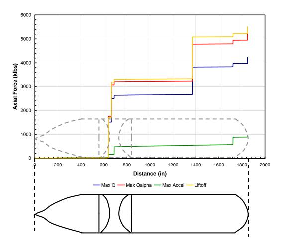
Figure 18. Axial Load Magnitude Variation along the ET for each Load Condition.
