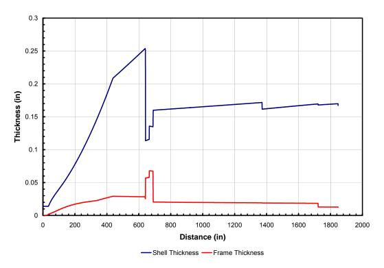
Figure 20. Shell and Frame Thickness Variation along the ET.
