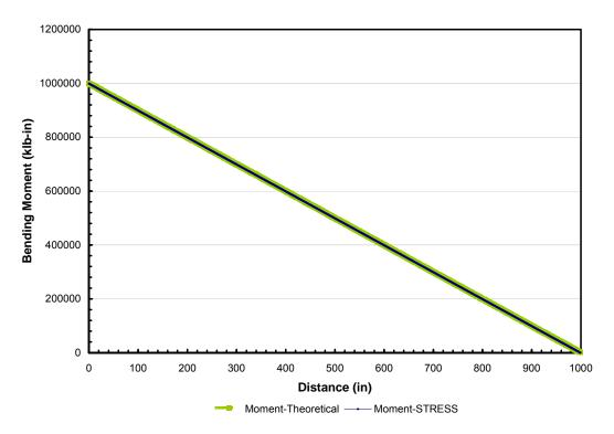
Figure 7. Bending Moment Accuracy of Discretized vs. Theoretical Method for End Loaded Cantilevered Beam
