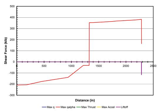
Figure 28. Shear Force Variation along the Fuselage for each Load Condition of the EELV
