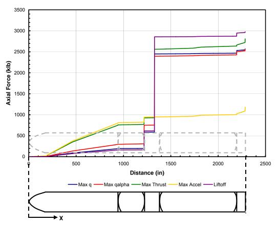
Figure 17. Axial Load Magnitude Variation along the EELV Fuselage for each Load Condition.
