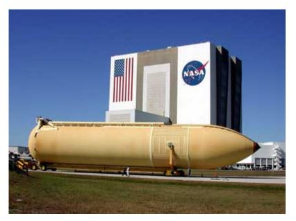
Figure 16. Space Shuttle External Tank.
