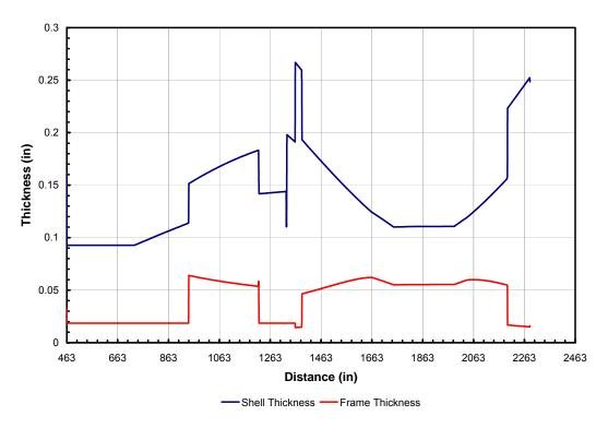
Figure 19. Fuselage Shell and Frame Thickness Variation along the EELV.
