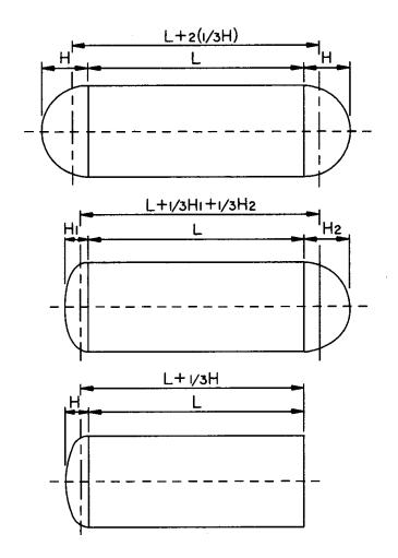
Figure 3. Effective Length of Cylindrical Tanks with Various End Closures (Jawad, *Design of Plate & Shell Structures*, p. 376).
