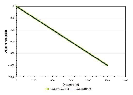
Figure 8. Axial Force Accuracy of Discretized vs. Theoretical Method for Uniform Loaded Cantilevered Beam
