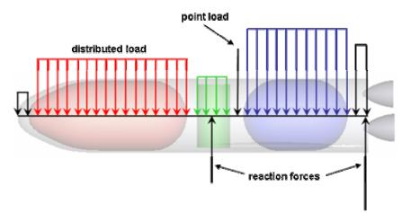
Figure 2. Visual Representation of Vehicle Weight Definition.
