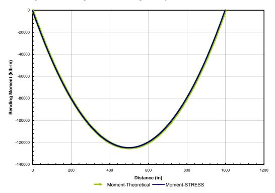
Figure 6. Bending Moment Accuracy of Discretized vs. Theoretical Method for Uniformly Loaded Simple Support Beam
