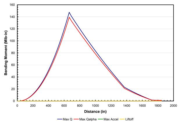
Figure 32. Bending Moment Variation along the Fuselage for each Load Condition of the ET
