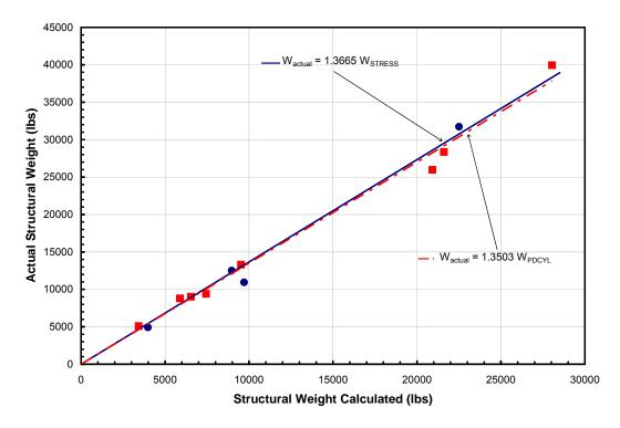
Figure 23. Regression Comparison of Structural Weight Results from GT-STRESS and PDCYL.
