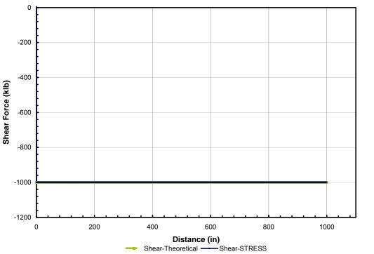
Figure 4. Shear Force Accuracy of Discretized vs. Theoretical Method for End Loaded Cantilevered Beam
