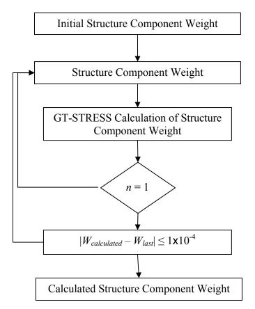
Figure 13. Convergence Process for Determining Structure Component Weight.
