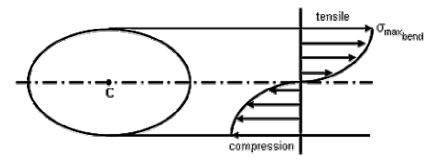
Figure 10. Bending Moment Distribution over an Elliptical Section
