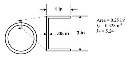
Figure 12. Shape and Dimensions of Frame Cross Section.
