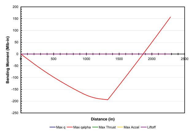
Figure 29. Bending Moment Variation along the Fuselage for each Load Condition of the EELV
