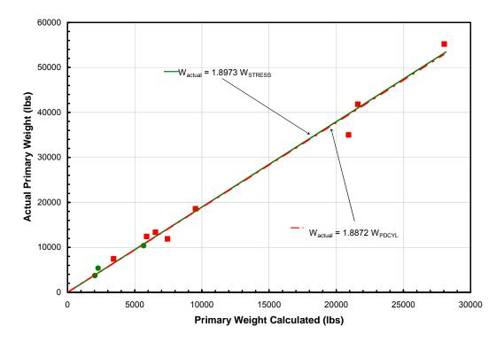
Figure 24. Regression Comparison of Primary Weight Results from GT-STRESS and PDCYL.
