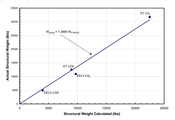
Figure 21. Linear Regression of Structural Weight.
