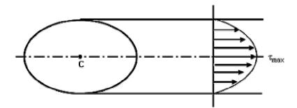
Figure 9. Shear Stress Distribution over an Elliptical Section
