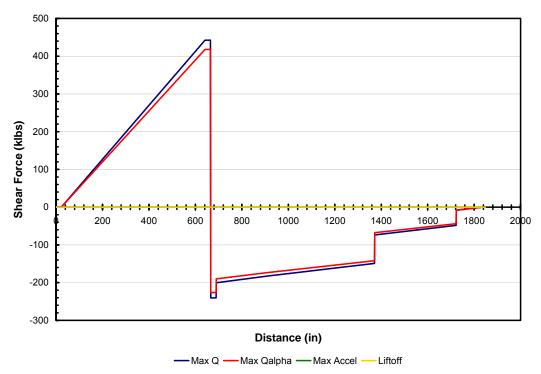
Figure 31. Shear Force Variation along the Fuselage for each Load Condition of the ET
