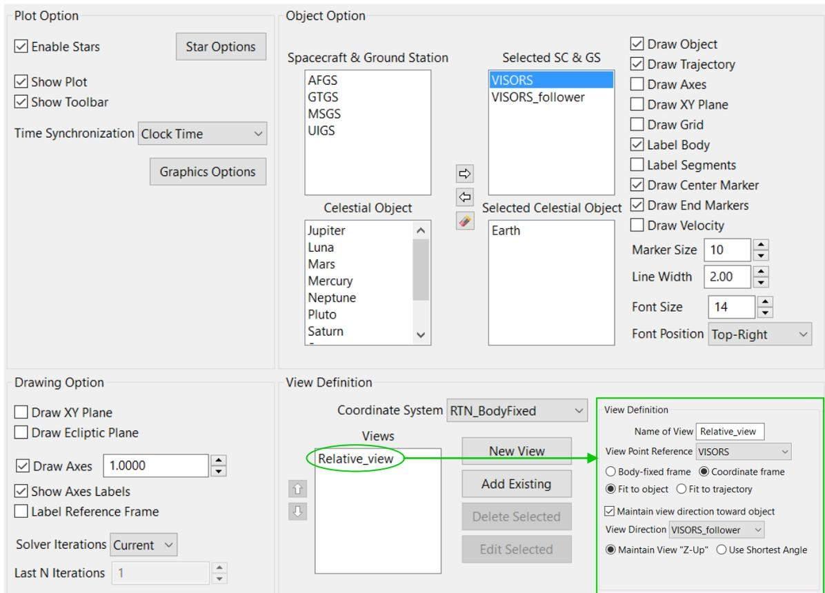
**Fig.1 GMAT tool configuration for the Bodyfixed relative view**
