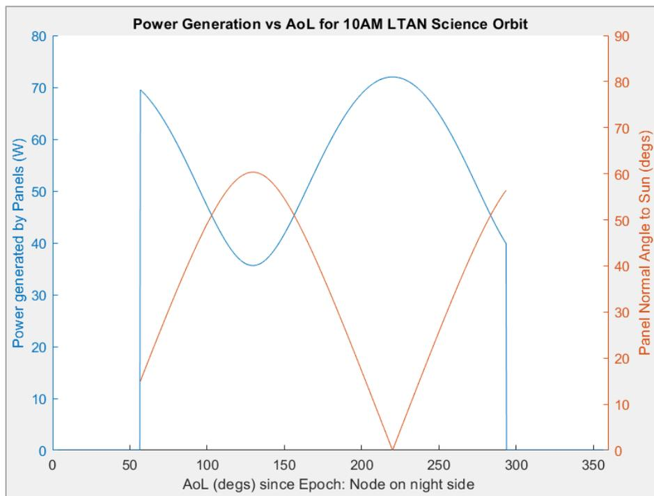
Fig.11 Science orbit power generation for a RAAN of  $329.56^\circ$  (nominal case)
