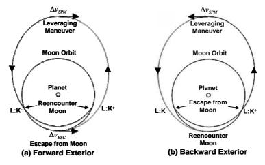
Figure 2 Exterior  $V_{\infty}$  Leveraging Maneuver Geometry
