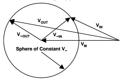
Figure 3 Two-Body Zero-Point Patched Conic Velocity Diagram
