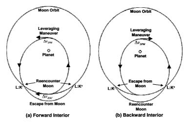
Figure 1 Interior V<sub>∞</sub> Leveraging Maneuver Geometry
