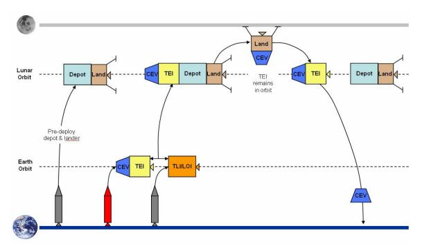
Figure 6. Diagram of Reusable Lunar Architecture.
