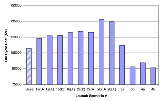
Figure 25. Life Cycle Cost for Launch Vehicle Trade Study (Reusable Architecture).
