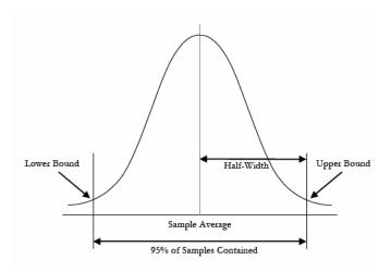
Figure 2. Probability Density Function of a Normal Distribution.
