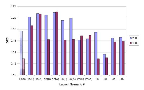
Figure 37. Overall Evaluation Criterion (Cost, Reliability, and LEO Time) for TLI Trade Study (Expendable Architecture).
