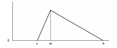
Figure 1. Probability Density Function of a Triangular Distribution.
