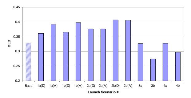
Figure 28. Overall Evaluation Criterion (Cost and Reliability) for Launch Vehicle Trade Study (Reusable Architecture).
