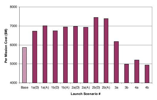
Figure 26. Cost Per Mission for Launch Vehicle Trade Study (Reusable Architecture).
