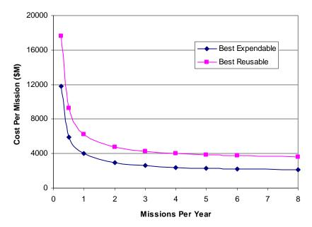
Figure 44. Cost per Mission as a Function of Annual Flight Rate.
