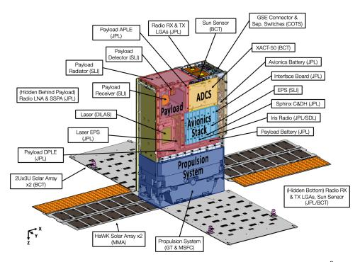
Figure 1: Lunar Flashlight spacecraft overview and body frame axes.<sup>3</sup>
