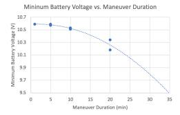
Figure 10: Minimum battery voltage reached during off-sun maneuvers.
