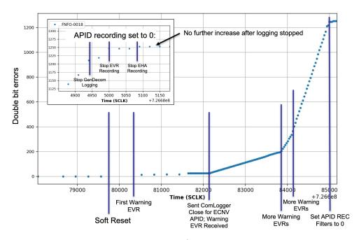
Figure 21: Double bit errors on /eng partition during anomaly.
