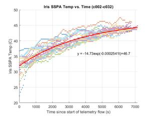
Figure 14: Iris SSPA temperatures across multiple contacts.
