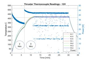
Figure 7: Catalyst bed heating curves from LFPS I&T.<sup>10</sup>
