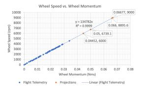
Figure 11: Correlation of reaction wheel speed and computed momentum telemetry.
