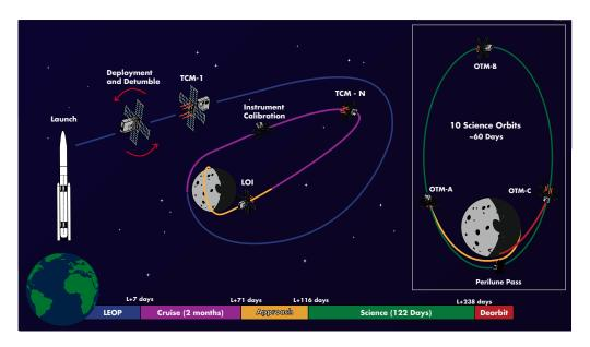
Figure 2: Concept of operations for the Lunar Flashlight mission.
