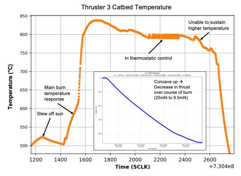
Figure 19: Synthesized temperature and Doppler data used to assess maneuver performance.
