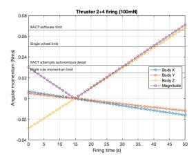
Figure 12: Angular momentum change from firing two thrusters simultaneously.
