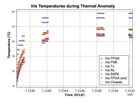
Figure 15: Iris temperatures during weekend 'hot' case.
