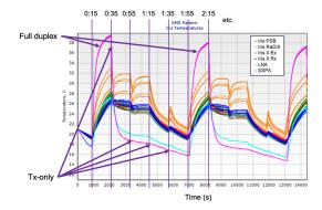
Figure 6: Thermal model simulation results of initial SMS radio configuration.
