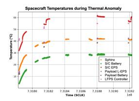
Figure 16: Additional spacecraft temperatures during weekend 'hot' case.
