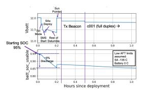
Figure 3: Power profile simulation of deployment and initial boot-up.
