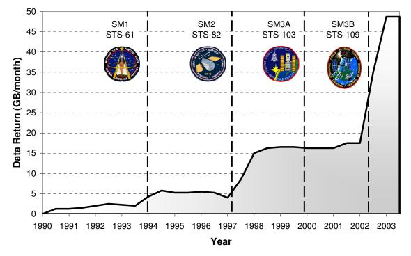
Figure 1. Hubble Space Telescope Data Return (adapted from Ref. 9).
