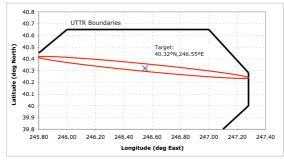
Figure 4: Nominal Landing Footprint (-3.45° Entry Flight Path Angle)
