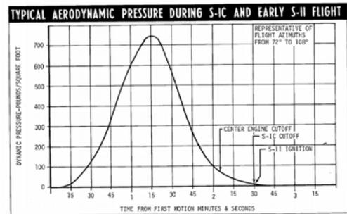
Figure 4 - Saturn V Dynamic Pressure versus Time<sup>6</sup>
