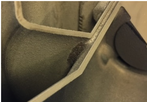
Figure 7: Example of Partial Fusion of Unsintered Powder
