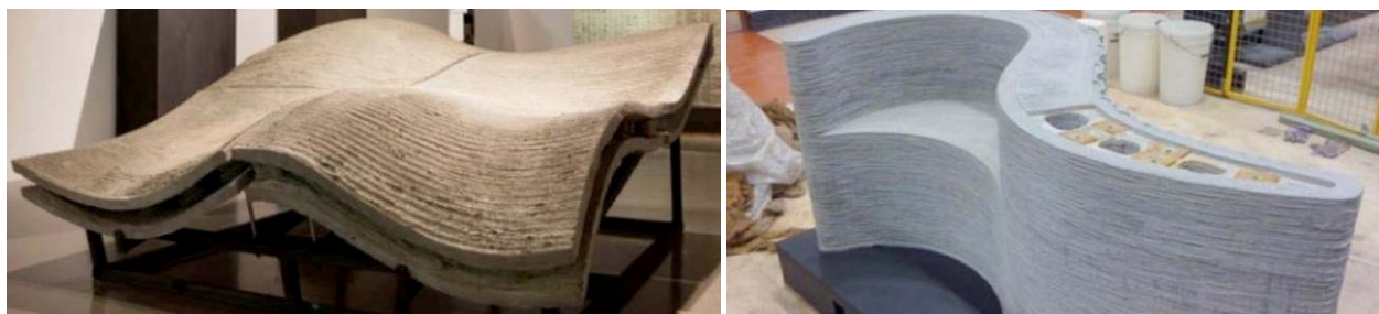
Figure 1. Free-form large scale concrete parts printed at Loughborough University (Le et al, 2012a; Le et al, 2012b; Lim et al, 2012)
