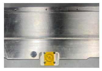
Fig. 14 EB weld of the pathfinder tank assembly
