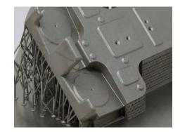
(b) Skipping line due to failure
