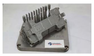
Fig. 12 One of the four flight-grade manifolds after L-PBF printing, Image Credit: Volunteer Aerospace
