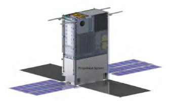
Fig. 1 Lunar Flashlight spacecraft, specifying the location of the propulsion system
