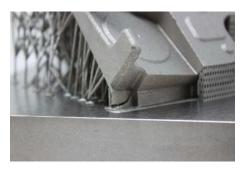
(a) Support material failure
