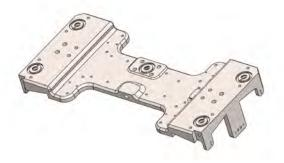
Fig. 7 CAD of the Lunar Flashlight manifold
