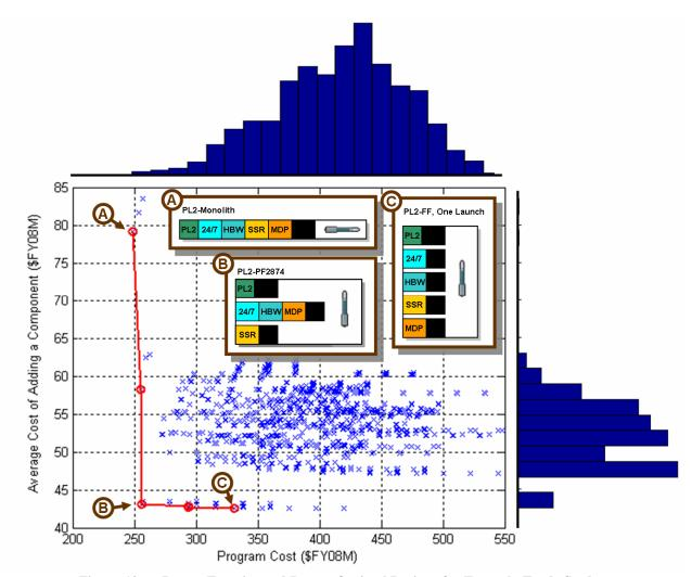
**Figure 12.** Pareto Frontier and Pareto-Optimal Designs for Example Trade Study. Here, each blue "x" represents one of 3190 possible designs, the red circles indicate the non-dominated designs, and the red line indicates the interpolated Pareto frontier. Three interesting designs are noted by the letters A, B, and C.
