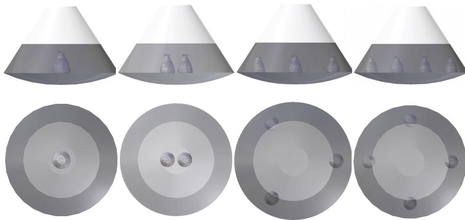
**Figure 7: Engine configuration options for 15 m diameter vehicle.**
