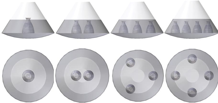
**Figure 6: Engine configuration options for 10 m diameter vehicle.**
