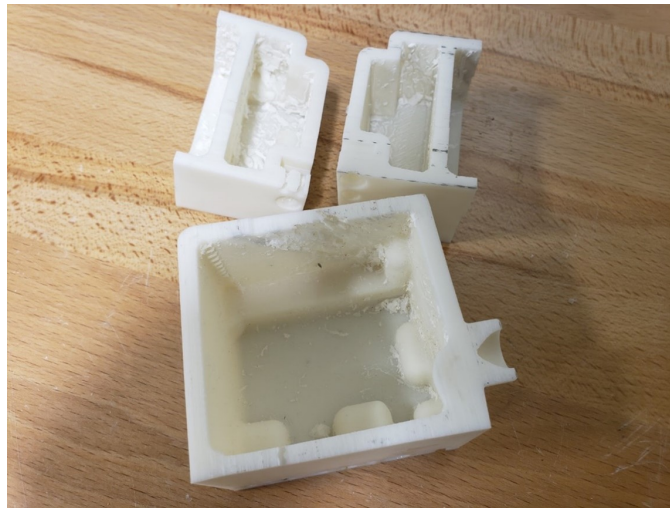
Figure 2 Cutaway view of SWARM-EX propulsion system printed structure prior to cleaning.
