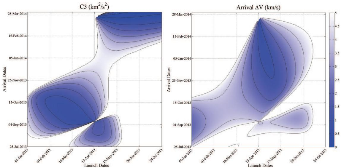
**Figure 1. Standard pork chop plots of launch C3 and hyperbolic arrival velocity. Note that for this asteroid problem, arrival velocity is equivalent to arrival  $\Delta V$  since the spacecraft is required to come to a complete stop relative to the asteroid.**
