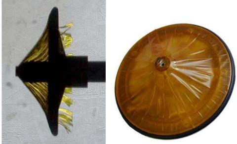
Fig. 2: Profile and deformed shape of model during (left) and after (right) testing.
