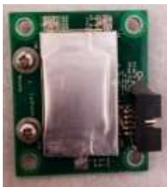
Figure 29 Laser Driver Board Capacitor
