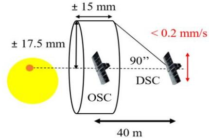
**Figure 2. Relative position/velocity requirements imposed on formation during observation.**
