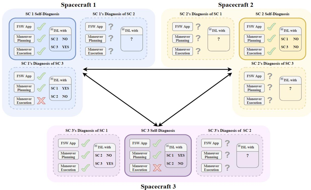
**Figure 6. Formation statuses sharing scheme across a formation of three spacecraft.<sup>10</sup>**
