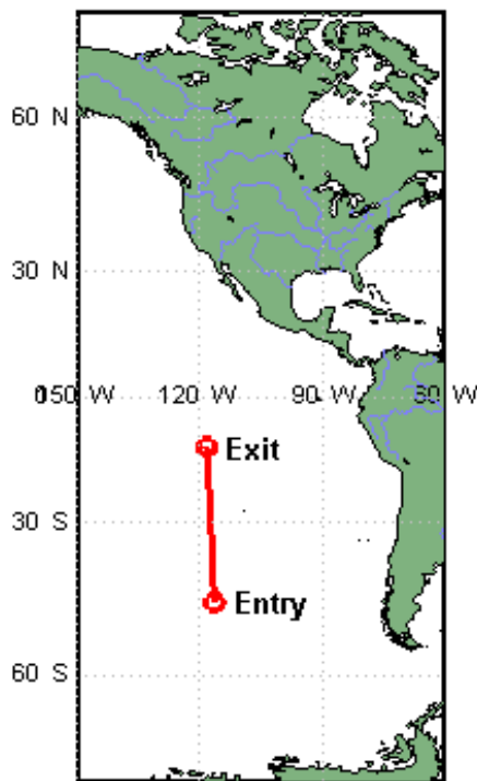
Figure 4. Representative ground track for Orion lunar return aerocapture into LEO.
