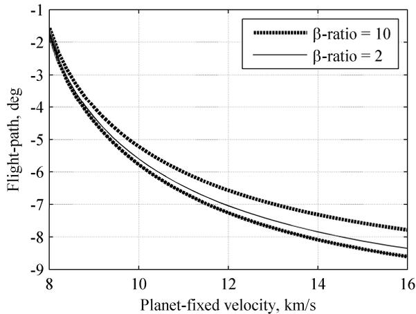
**Figure 5 - Flight-path angle corridor at Earth**
