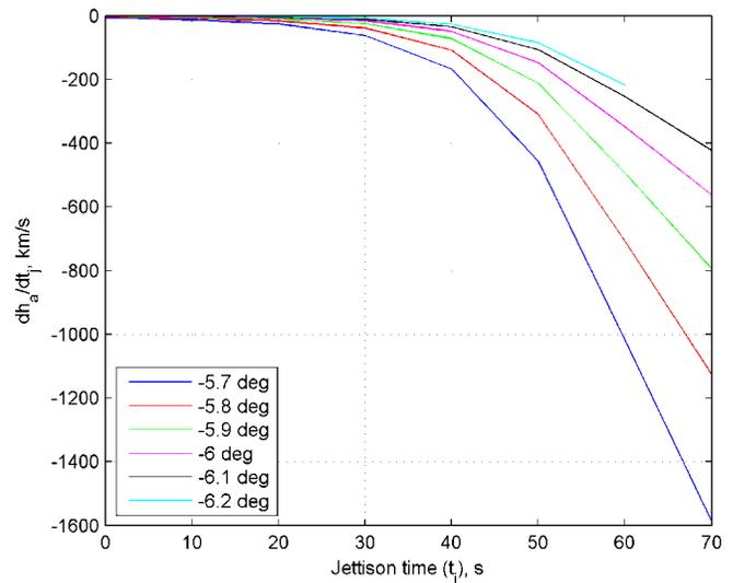
**Figure 12 - Sensitivity of final apoapsis altitude to jettison time at Earth at 11 km/s**
