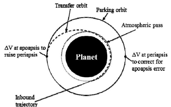
**Figure 1 - Aerocapture maneuver to a low parking orbit**
