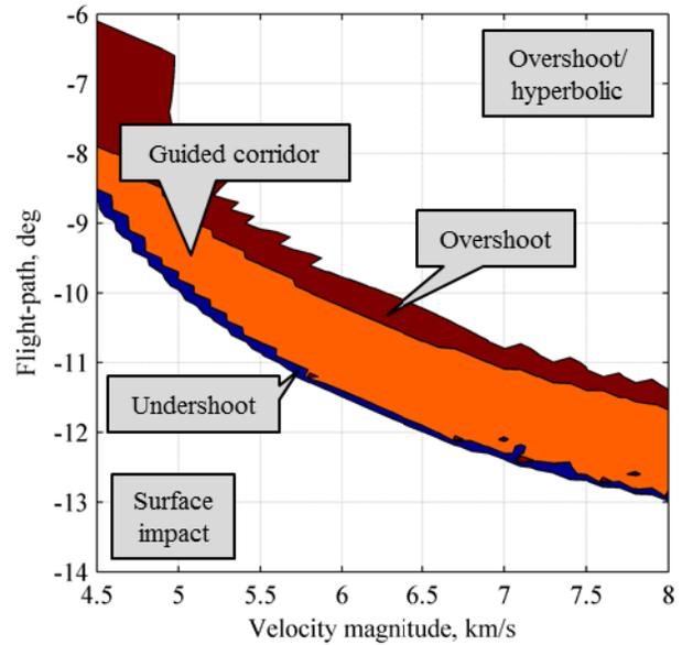
**Figure 14 - Guided flight-path corridor at Mars for single-event jettison configuration**
