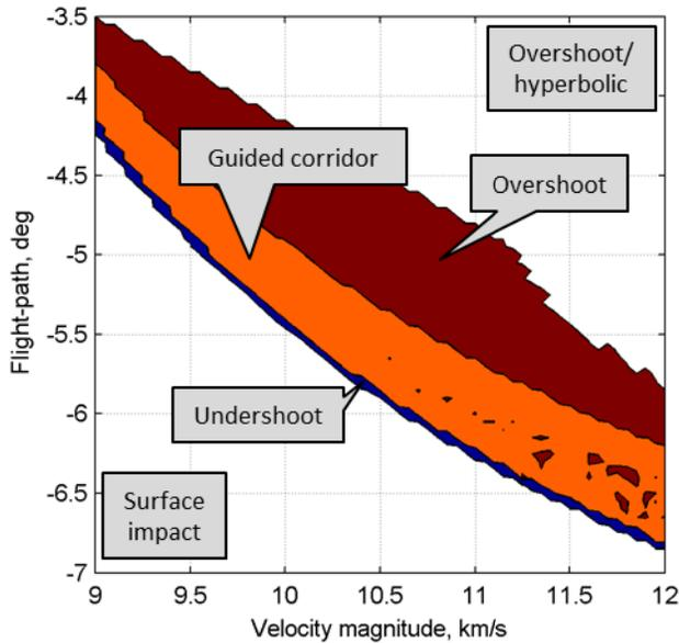
**Figure 13 - Guided flight-path corridor at Earth for single-event jettison configuration**
