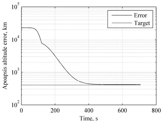
**Figure 11 - Apoapsis error during aerocapture at Earth**
