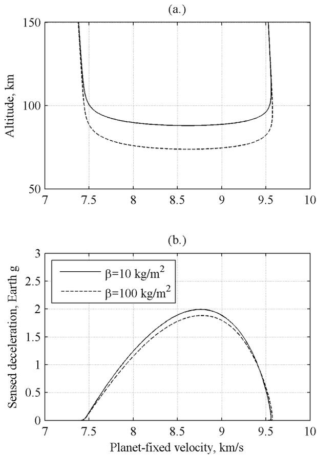
**Figure 4 – Corridor-bounding trajectories for aerocapture at Earth: (a.) altitude and (b.) deceleration**
