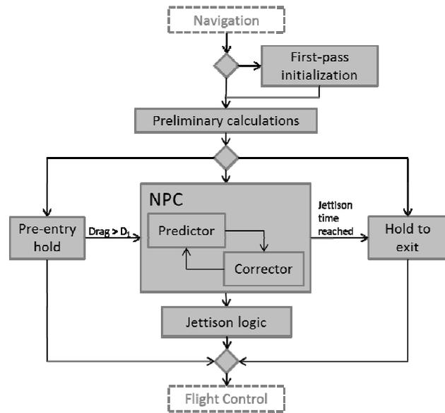
**Figure 9 - Single-event jettison guidance algorithm block diagram**
