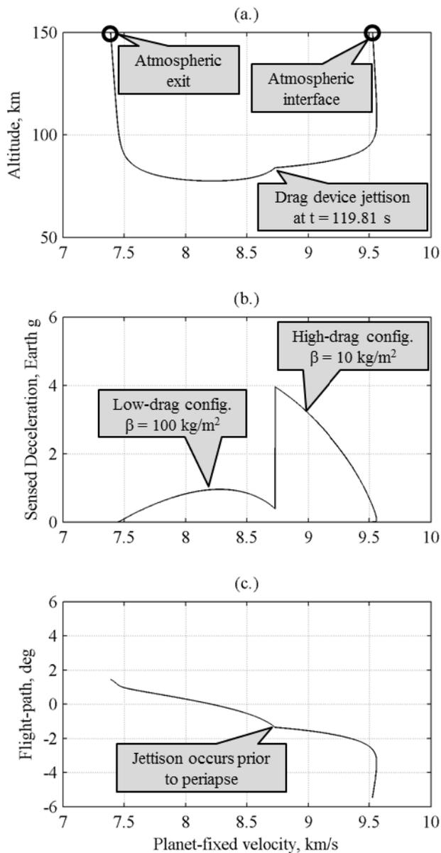
**Figure 10 - Sample guided aerocapture trajectory at Earth**
