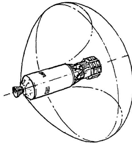
**Figure 3 - Drag coefficient modulation AOTV concept [5]**
