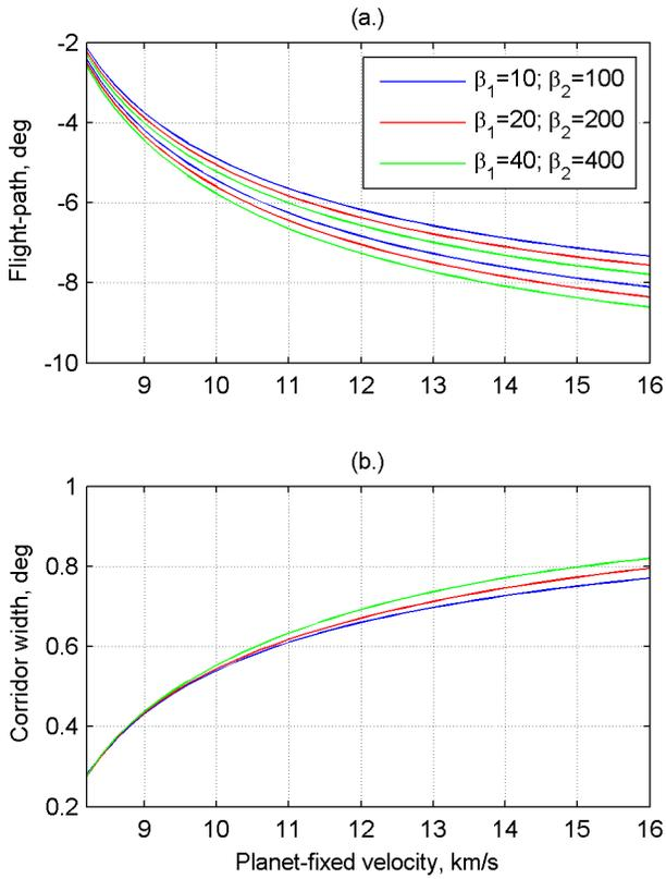
**Figure 8 - Flight-path corridor (a.) and width (b.) for several  $\beta$  magnitudes at Earth**
