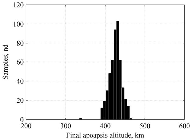
**Figure 15 - Final apoapsis altitude at Earth for a nominal velocity and flight-path of 10 km/s and -5.2 deg**
