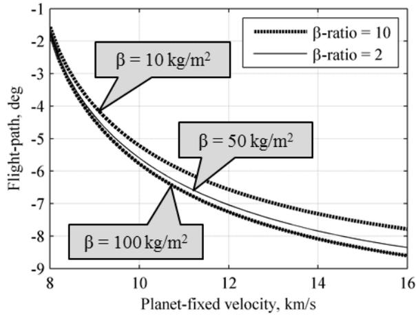
**Figure 7 - Flight-path angle corridor at Earth for two different  $\beta$ -ratios**
