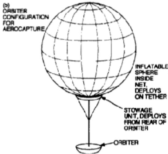
**Figure 2 - Trailing thin-film ballute system concept [1]**
