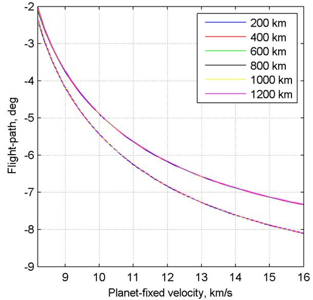
**Figure 6 - Flight-path corridor as a function of velocity for several apoapsis altitude targets at Earth**
