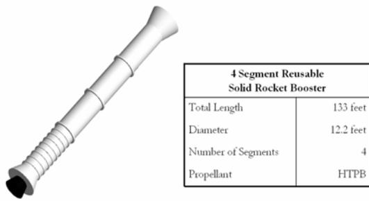
Figure 5. 1<sup>st</sup> Stage Configuration RSRB.
