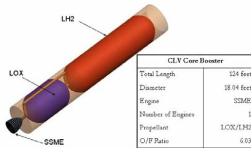
Figure 6. 2<sup>nd</sup> Stage Configuration (SSME).
