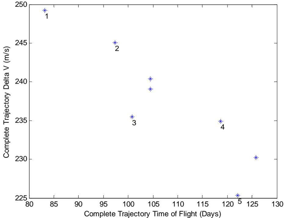
**Figure 6 Complete Trajectory Scatter Plot for Ganymede-Europa (6:5-5:6) Transfer**
