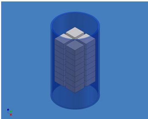
Figure 13 – Standard MMRTG Casing Holding Four Times the GPHS Units
