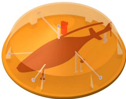
Figure 11 – Helicopter Inside Aeroshell
