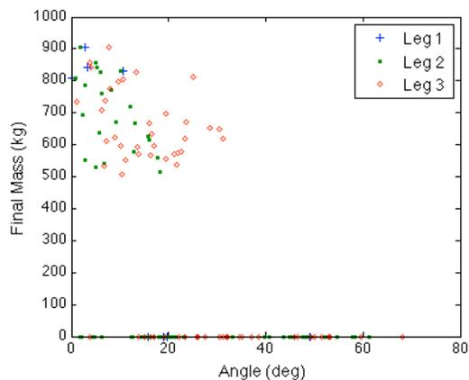
Fig. 4: Maximum low-thrust final mass as a function of the angle between the angular momentum vectors for each asteroid pairing.
