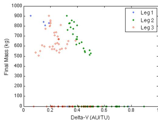
Fig. 5: Maximum low-thrust final mass as a function of the optimal, two-impulse, phase-free  $\Delta V$  for each asteroid pairing.
