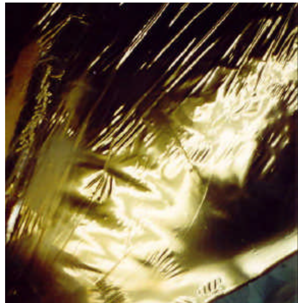
Figure 7: Inflatable reflector surface in mid-heating process. Note the wrinkles in some areas where the mylar hasn't been shrunk yet.
