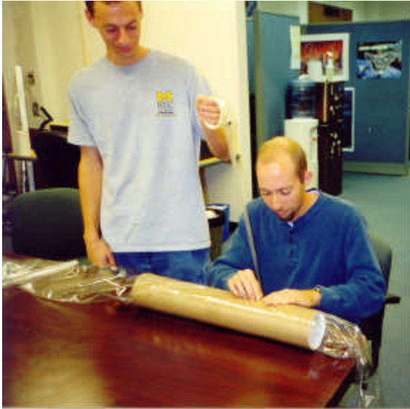
Figure 8: The struts and support tube are carefully wrapped around a mandrel and taped together.
