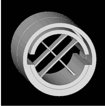
**Figure 4: CAD image of a flex pivot**
