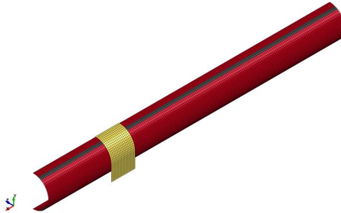
Figure 6: CAD model for Four-point Bend Test Simulations
