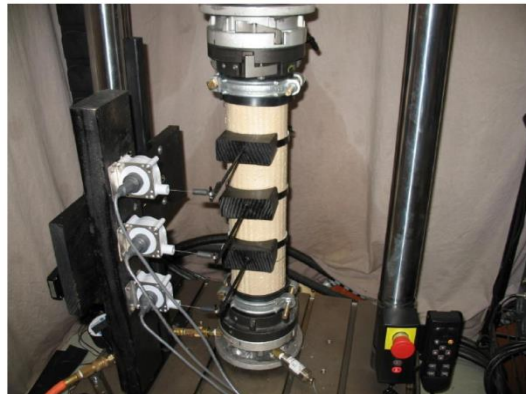
Figure 5: Torsion and Tension Test Setup 17
