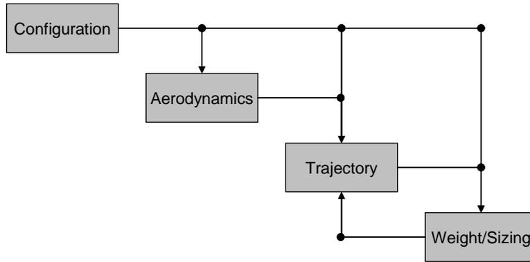
**Figure 6. Launch Vehicle Design Structure Matrix**
