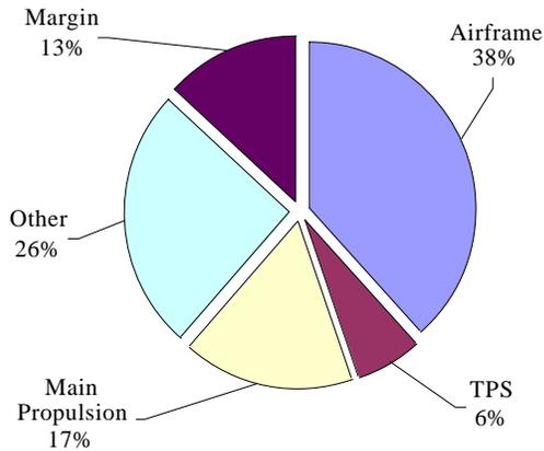
**Figure 14.** *Hyperion* Dry Weight Breakdown.
