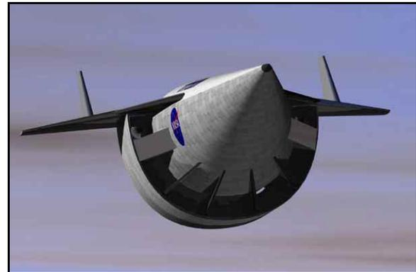
Figure 3. Hyperion Loiter with Ducted Fans.
